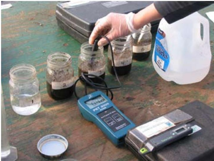
**Figure 1.1** - This picture shows a pest manager testing electrical conductivity (EC) in container production. The EC of a medium is directly related to the concentration of ions it holds, so a higher EC reading means there are more ions in the medium. Since plants can only take up ions, a higher EC means there are more elements available to the plant.
