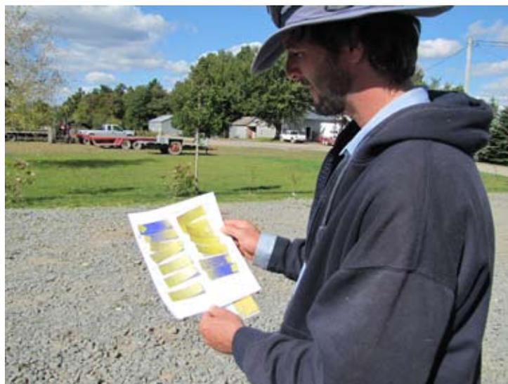
**Figure 6.1** - Water sensitive paper is great for evaluating how your sprayer works in the field. By setting pieces of water sensitive paper in different places among the plants you spray, you can see where your spraying equipment is successful.
