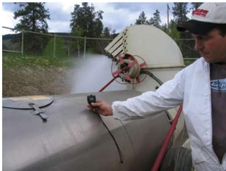
**Figure 5.3** - Calibrating your sprayer is an easy thing to do, and can save you a lot of aggravation. Calibrating is a good way to determine how your equipment is functioning compared to how it is supposed to function, and to identify small problems that may turn into big ones if not addressed early.
